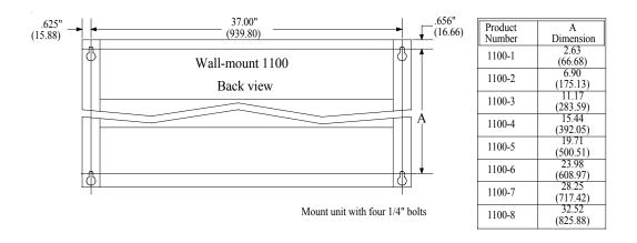
Figure 15. Mounting dimensions for wall-mount PMD 1100s
