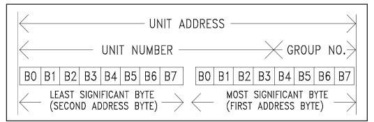
Figure 11. Unit Address Byte Designation
