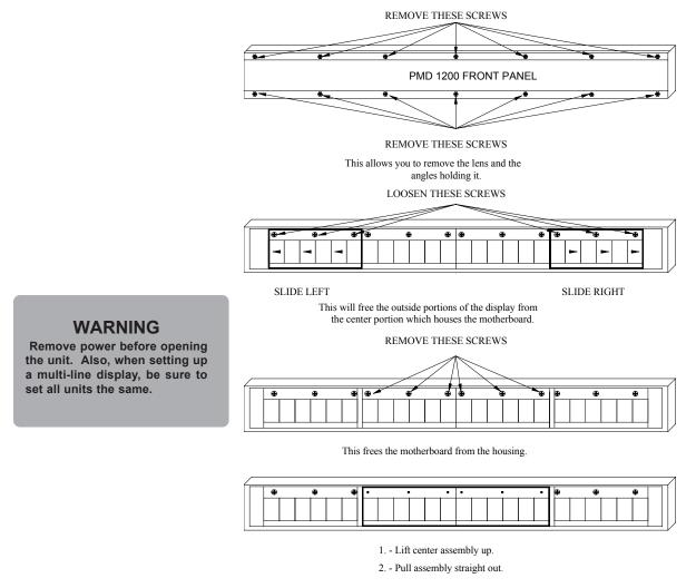
When reassembling the unit, be sure to get all the pins aligned while sliding the outside boards in.
