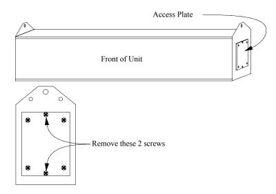
Figure 2. Opening the access panel
