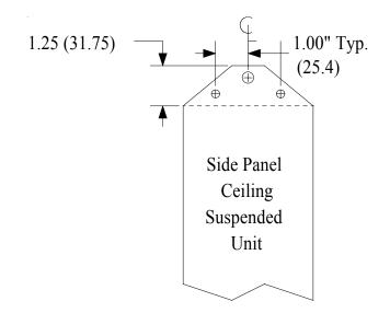
Figure 14. Mounting holes for ceiling-suspended units
