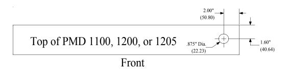
Figure 18. Cable routing hole location
